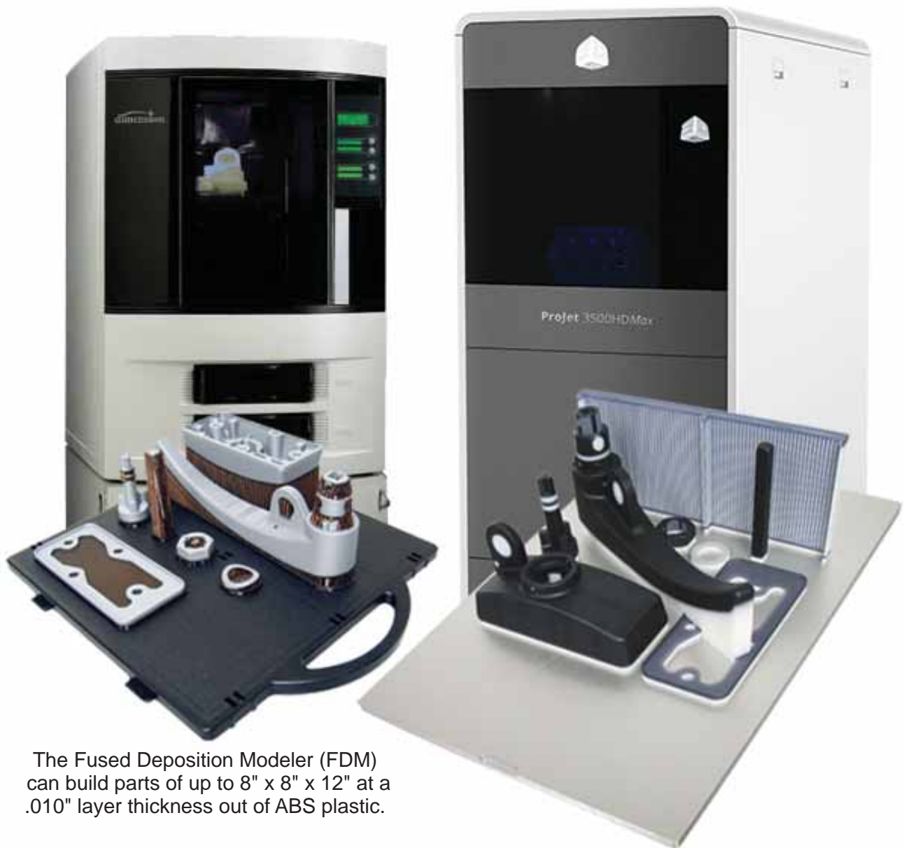
The Multi-Jet Modeler (MJM) can build parts of up to 11.75" x 7.3" x 8" at a .001" layer thickness out of Acrylic plastic.
